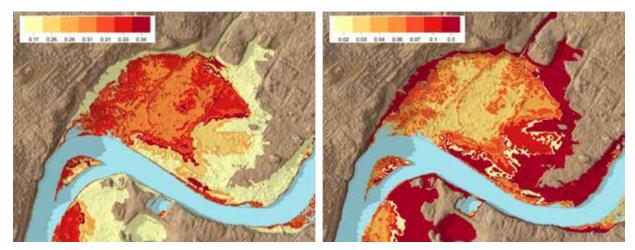
Figure 11: Mean contributions to flood levels in the wetland from tidal and river flooding
