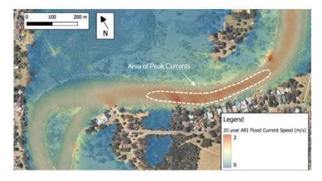
Figure 18: 20-year ARI flood current speeds (BMT WBM 2018)
