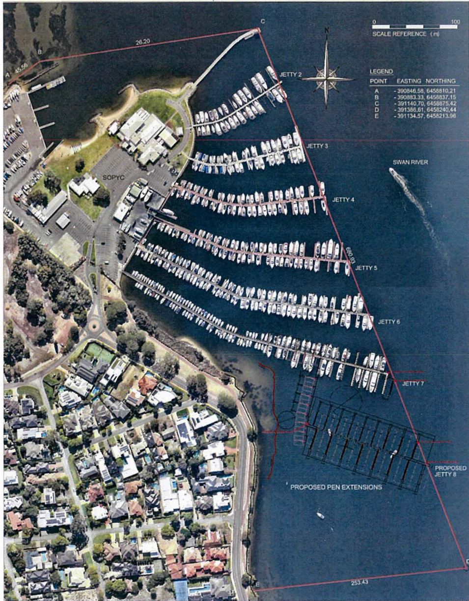
Figure 1: Existing marina with proposed finger jetty 8 (River reserve lease area shown in red)
