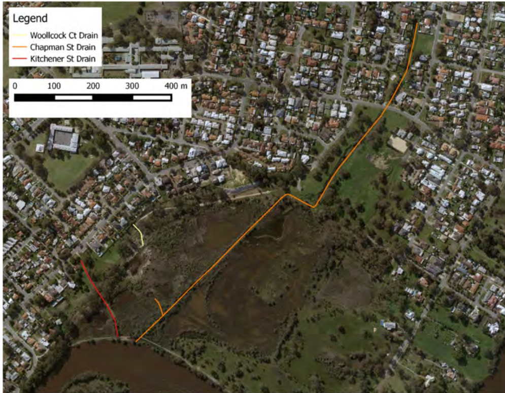
Figure 3: Open drains discharging to or draining through the Reserve.
