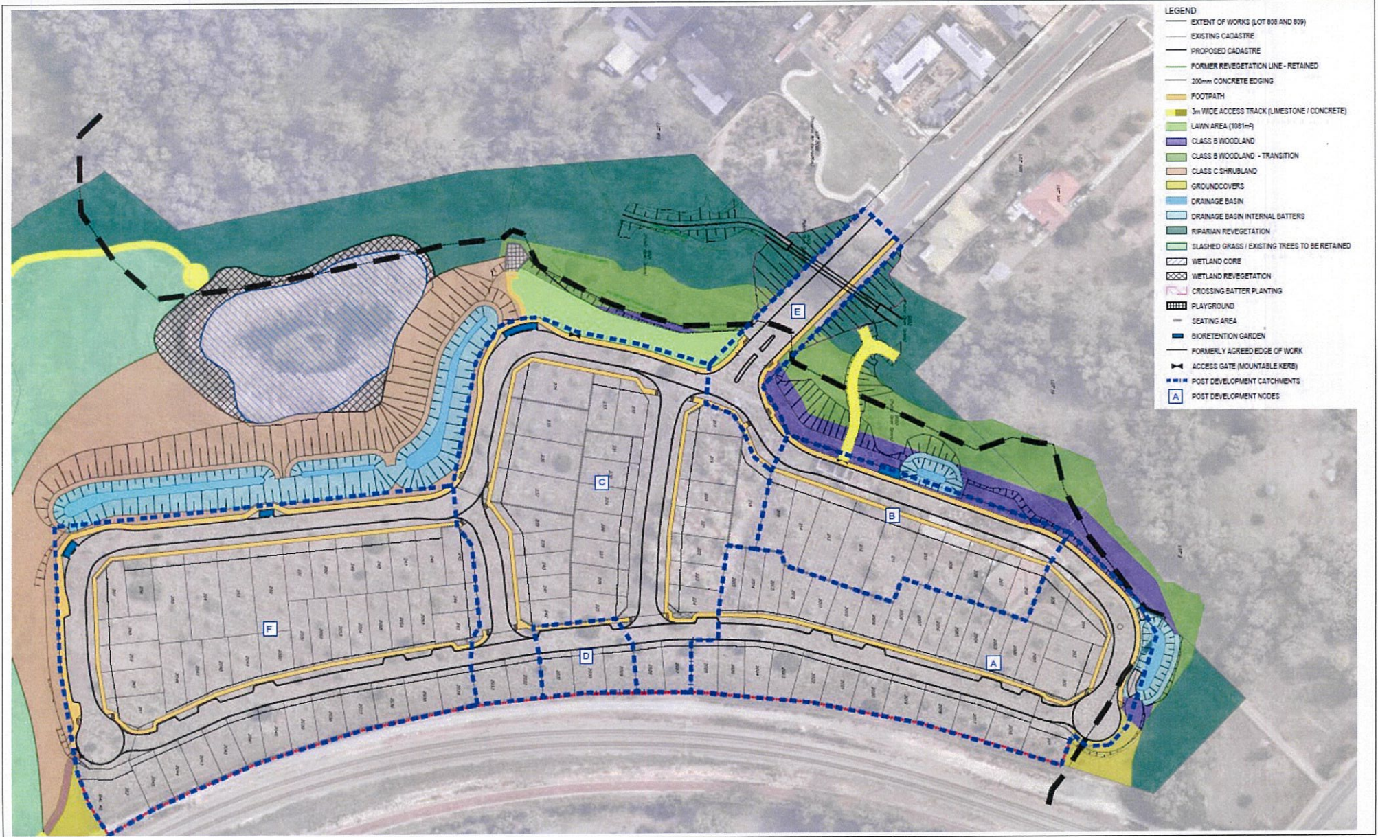
Figure 11 Post Development catchments
