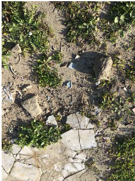
Photo 16. Typical suspect ACM scatter (G63).
