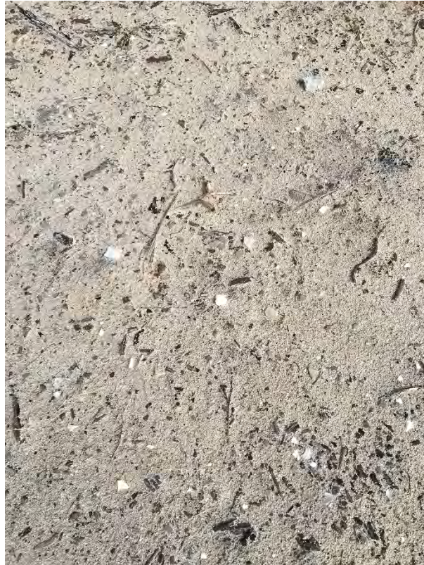
Photo 21. Typical suspect ACM scatter on tracks (G43).
