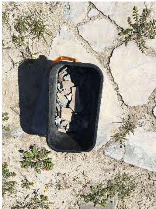
Photo 18. Suspect ACM fragments collected at G63.
