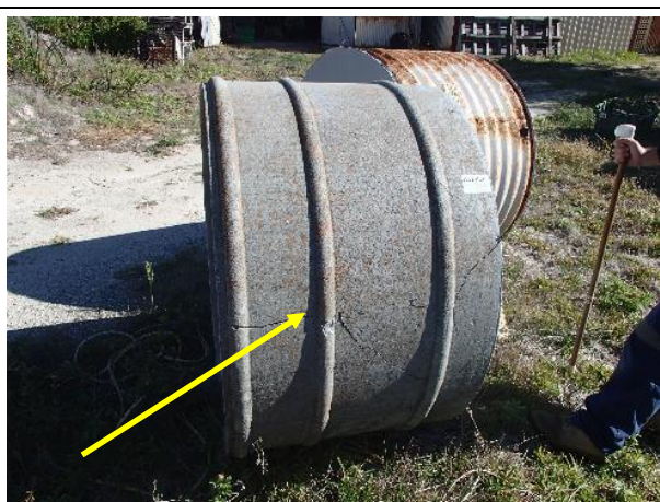
Asbestos cement soak well. External to Shack W41.
