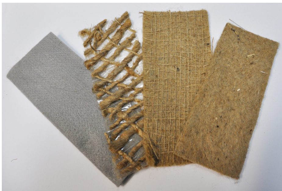
Figure 3 Erosion control matting commonly used in foreshore restoration projects in the Swan Canning Riverpark, from left Bidim® geofabric, coir mesh/coir netting, fine jute mat and thick jute mat
